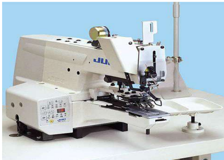
Stitching machine: This machine is used for stitching pads for the interior of helmet.
