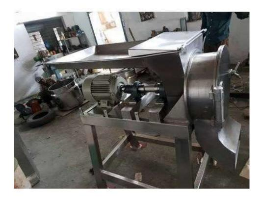
➤ Mixing Machine: This machine can be used to mix processed garlic with the required ingredients such as spices, oil, butter etc.
