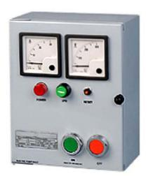
**Working of motor starter Panel:** Motor starters consist of two devices—a contactor that completes the circuit to the motor and an overload relay that monitors the current the motor is drawing. This overload protection device is set to a predetermined maximum load that the motor can safely handle. When a condition occurs that causes the motor to exceed the
