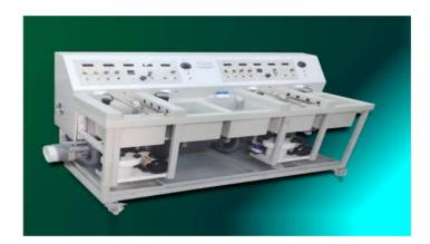
➤ Electroplating Machine: Electroplating is basically the process of plating a metal onto the other by hydrolysis mostly to prevent corrosion of metal.
