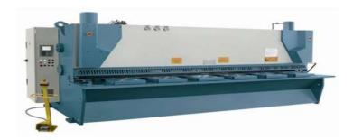
> Shearing machine: The workpiece is fixed in the machine tool and subsequently cut by pressing a blade through the workpiece and into a die underneath. Unlike many other processes, shearing does not use a rotating tool-piece. Instead, it works like a pair of scissors which means a blade presses against it using a good amount of force.
