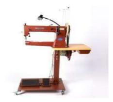
**Pressing Tool Machine:** This is used to flatten the areas and edges around the bags.
