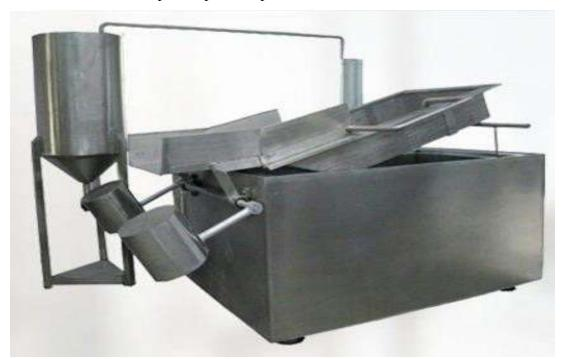
**Seasoning tumbler:** A machine that plays a vital role in salting and seasoning large quantities of Kurkure type snacks and other snacks with a gentle, effective tumbling action. Variable speed control and adjustable tilt produce a uniformly covered product with minimal breakage and wastage.
