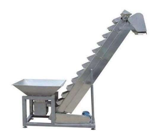
**Belt conveyor:** Belt conveyors are one of the most basic instruments in the food processing industry, and they're most widely used to transport bulk materials.
