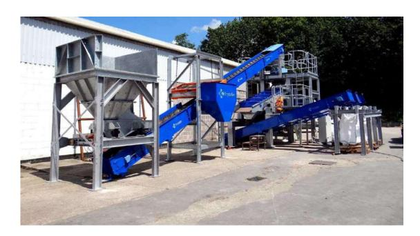
**Packing machine:** A bagging machine can be used to pack the finished product.
