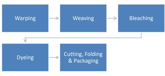
Fig. 1 – Process Flowchart
