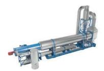
The rotary drum dryer is a hot air type of dryer, which dries objects in between 90 to 95 % dry solids. The material is gently dried as it cascades through the hot air flow.
