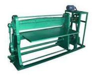
It's used to slice the given veneer sheet into items of required dimensions.
