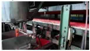
It's a specialized conveyor with perforated belt so as to hold particular type of material or to drain unwanted liquid.
