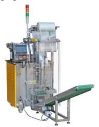
This machine counts the small unit load and packs it into single large unit after fixed count set by its controller.
