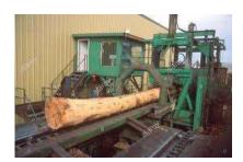
It's a machine which is used to remove bark from the tree logs utilizing appropriate cutters and mechanism.
