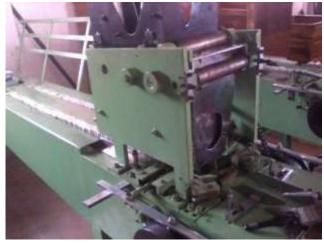
This machine is used to fill the matchstick into the boxes in appropriate quantity.
