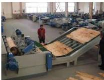
It's a machine designed to peel the debarked log into an appropriate thickness veneer sheet.
