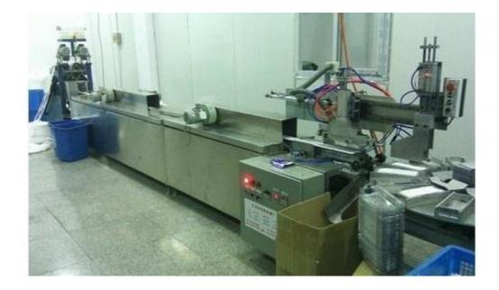
This machine is a special purpose machine specifically designed to manufacture cotton swabs without any adhesive, utilizing high speed tension winding.
