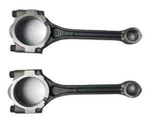
The connecting rod is constructed of forged steel and has an I-beam cross-section. Connecting rods are also made of aluminum alloy. To keep the engine balanced, they are perfectly matched in sets of comparable weight. Because the reciprocating weight is smaller, the lighter the connecting rod and piston, the higher the resultant power and the lower the vibration. The connecting rod transmits the power push from the piston to the crankpin, thus it must be extremely
