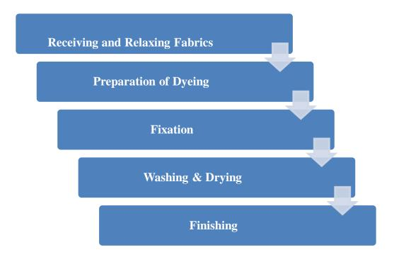
Fig. 1 – Process Flowchart
