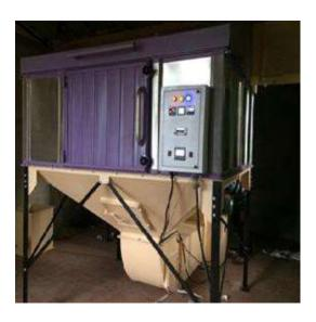
➤ Mixing Chamber: The mixing chamber are used to proper mixed coconut fibre with the latex before proceed for pressing process.
