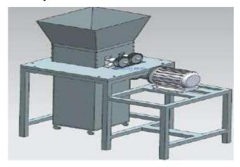
> Fiber Opening Carding Machine: The machine used to open treated fiber into loosed shaggy soft material.
