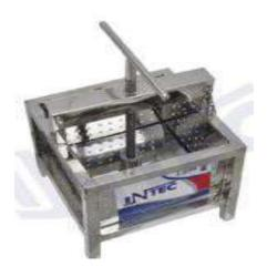
> Slice Cutting Machine: The slice cutting machine convert the partially semi liquid Cheese into a thin slice shape and remove moisture also during the process.
