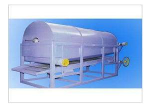
Air Screen Cleaner: This machine is used for the separation of undesirable material and seeds from desirable seeds in an air screen machine are done based on differences in seed size and weight. This removes the light seed and trash which was not removed by the upper air and the screens.
