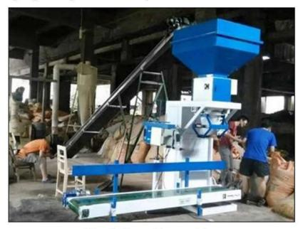
Fig.: Pellet packing machine
