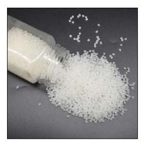
Fig.: Biodegradable PLA pellets
