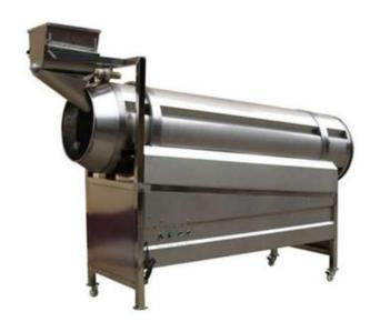
It's a simple rotating tumbler device used to apply seasoning and salt on given product, in this case namkeens.
