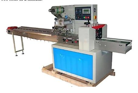
Fig.: Bandage packing machine
