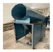
✓ Pulp bater: The pulp machine is used to convert the solid input product of banana tree into the semi liquid removing fibre from it.
