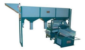
**Seed Destoner Machine:** This machine's aim is to remove stones and other mud material from the given grins.
