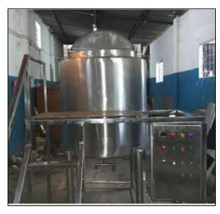
Fig.: Mixing tank
