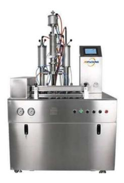
• Aerosol Propellant Filling Machine-If the product requires propellants or active ingredients, the aerosol feeding machine adds them. Only compressed gas is bottled here to be used for cleaning cameras and other equipment. The machine ispneumatically operated.
